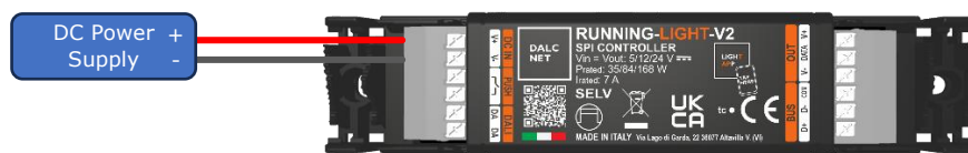
Figure 15: Power Supply Connection Diagram
