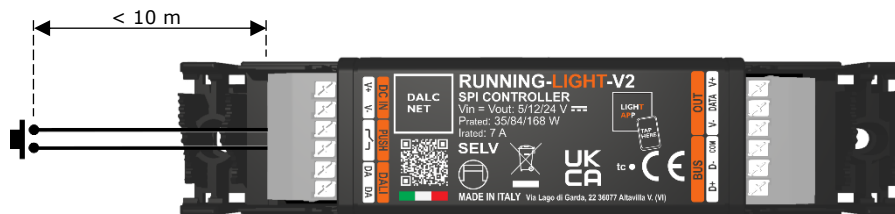
Figure 9: Local Control wiring diagram for Short Distances
