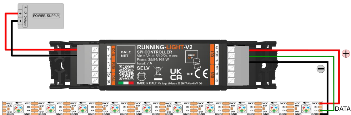
Figure 2: Connection diagram for Digital LED loads
