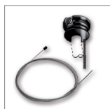
Retaining collar for cable 3 × 0.75 mm 2 or DALI cable incl. steel wire L = 1.5 meter for load up to 5 kg, for pendant light fixture
